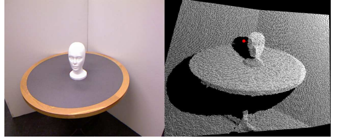
Fig. 4. Captured image from the Kinect RGB camera (Left) and point cloud representation of the same scene viewed from a slightly different angle (Right).
